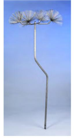
**APPLICATION:** For use wherever an air terminal (lightning rod) is appropriate and streamer delaying, or static dissipating qualities are desired. These dissipators are used in place of standard air terminals in a structural lightning protection system installed to UL-96A and NFPA 780 specifications. Terminal is mounted to the base most suitable to the structure on which it is being installed.
