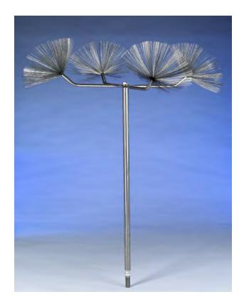
**APPLICATION:** For use wherever an air terminal (lightning rod) is appropriate and streamer delaying, or static dissipating qualities are desired. These dissipators are used in place of standard air terminals in a structural lightning protection system installed to UL-96A and NFPA 780 specifications. Terminal is mounted to the base most suitable to the structure on which it is being installed.
